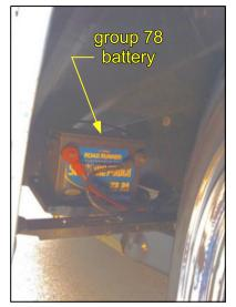
Battery is located behind right front wheel splash shield.
